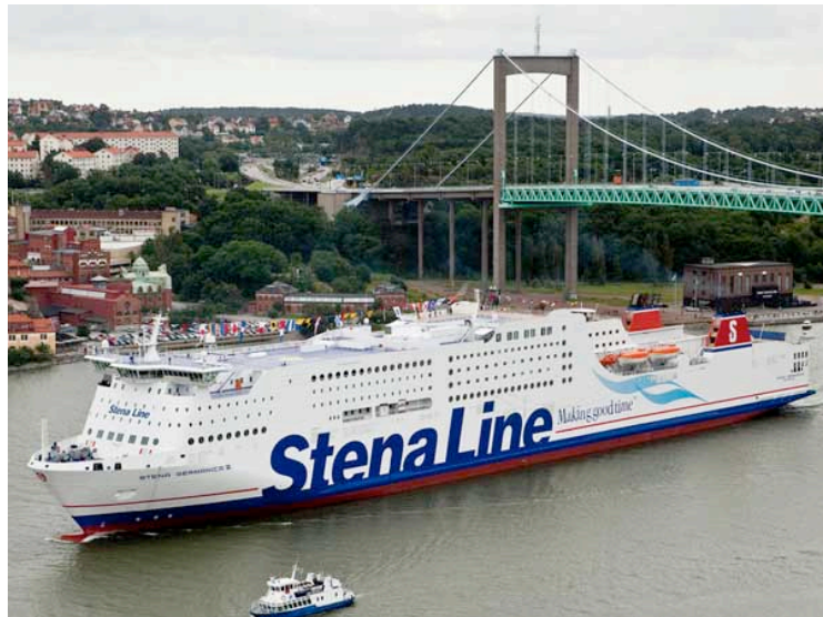
Figure 3: The Stena Germanica has Been Converted to Methanol
